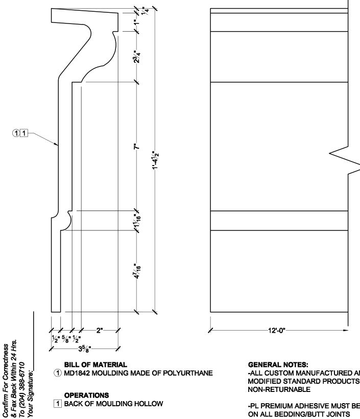
(1) MD1842 MOULDING MADE OF POLYURTHANE
